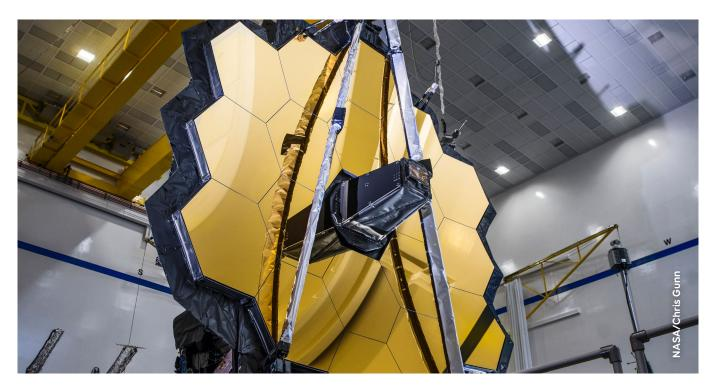
JWST after a deployment test of its primary mirror in the cleanroom.
