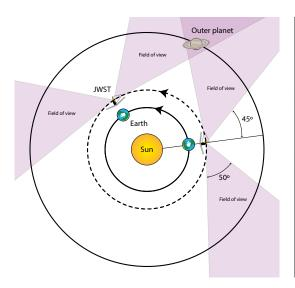
Figure 1: Mars and the outer planets of the Solar System come into JWST's field of view twice per year, when they are roughly at right angles to the Sun and the Earth.
