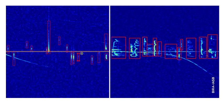
Left: Typical BRAMS spectrogram with mostly underdense meteor echoes. Right: BRAMS spectrogram obtained during a meteor shower with mostly overdense meteor echoes.
