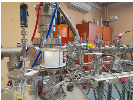
Figure 1. Setup prepared for the study of gases in ice. Ice samples was placed in a vessel connected to the newly commissioned ice chamber (left) equipped with a QMS. Bubbles of gas in the vessel during melting (right).
