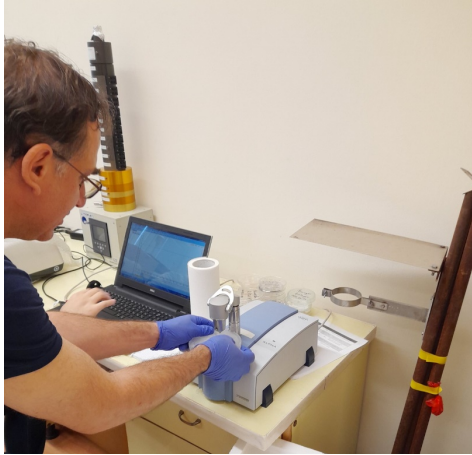
Figure 2. Sample of ice (3 cm thick) analysed with the ATR Bruker spectrometer.
