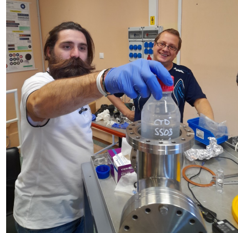
Figure 3. Placing the sample of sea water into the special vessel created at ATOMKI. The vessel was linked to the ice chamber and the QMS systems.
