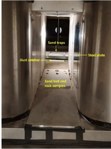
Figure 1. Experimental setup inside the wind tunnel.
