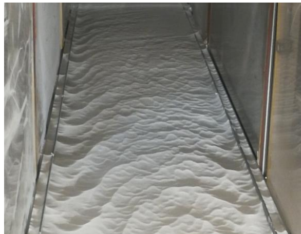
Figure 3 Example of hydrodynamic ripples produced on the simulated sandbed by high wind speed.
