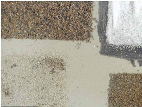
Fig. 1: Close up of the 4 different substrates. Clockwise from upper left: coarse regolith, glass beads, fine regolith, and regolith covered by dust.
