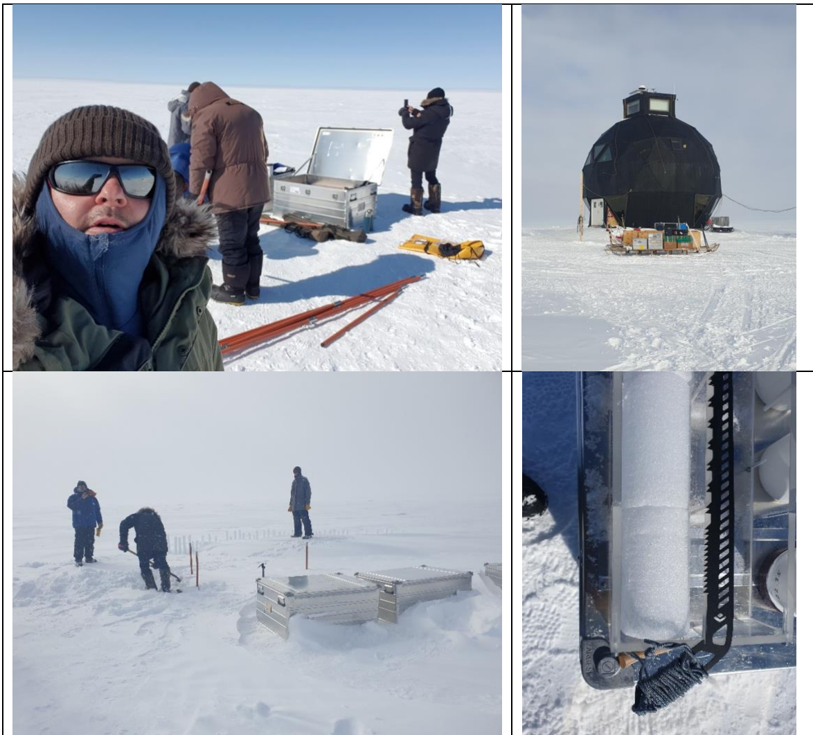
Figure 2. Drilling down to 24 m in the clean area of EGRIP (top left, bottom left); the main dome of EGRIP (top right); ice cores cut into subsamples of 15 cm.
