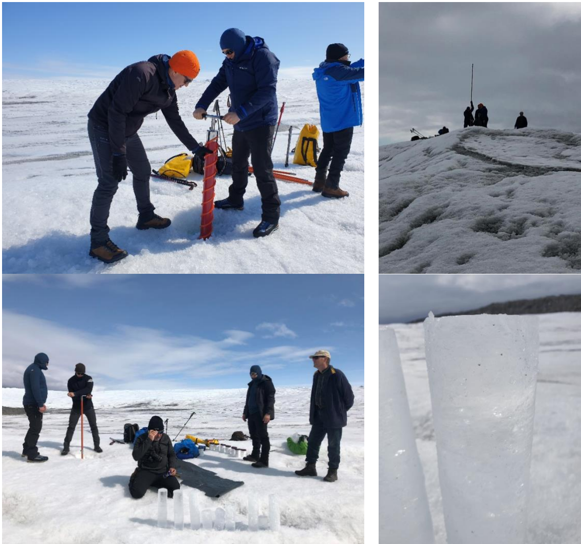
Figure 1. Drilling a shallow ice core at the ice margin close to Point 660 (top pictures and bottom left); and ice core entrapping some solid particles (bottom right).
