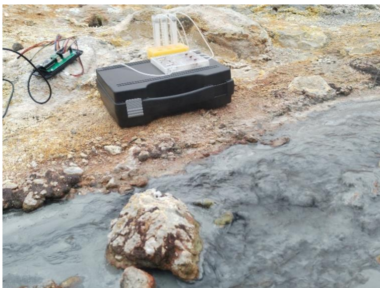
Figure 4: Image of the prototype developed by the team of researchers to perform in-situ, automated SERS analysis of liquid samples.
