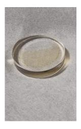
*Left*: example spectrum of the irradiated methanol sample, showing the formation of the usual radiolytic products such as CO<sub>2</sub>, CO, CH<sub>4</sub>, H<sub>2</sub>CO. *Right*: MgF<sub>2</sub> substrate with an organic residue resulting from the irradiation and warming up process.
