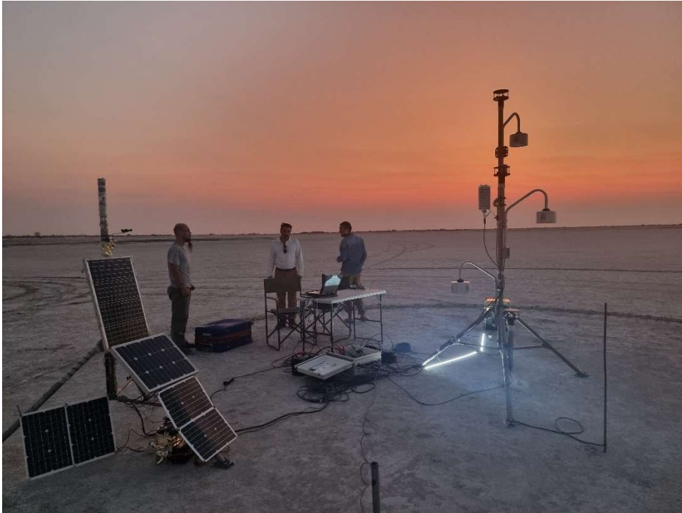
Fig. 1 On the left the mast with the solar panel and camera systems, on the right the main mast with the meteorological sensors.
