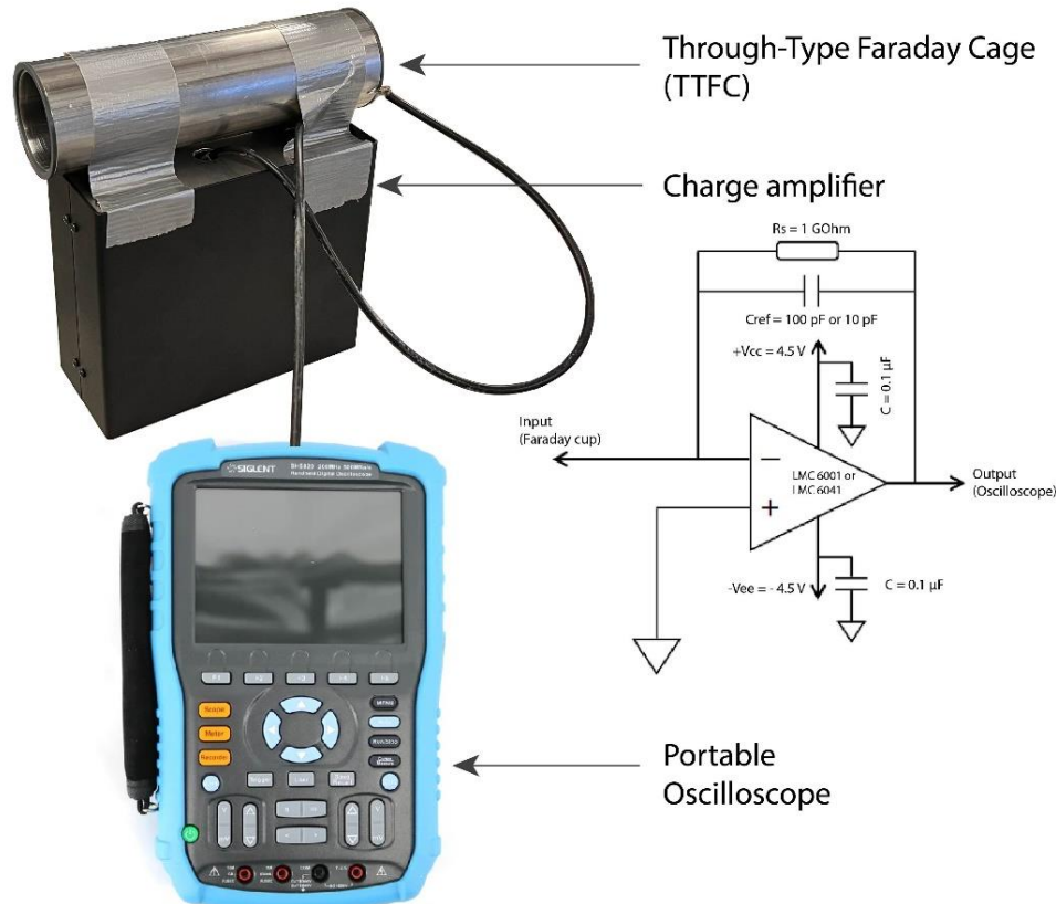
Figure 1 – Apparatus used for charge measurements. Here, the diameter of the TTFC is 5 cm and its length is 20 cm. The diagram describes the charge amplifier circuit, with the properties of each electrical component.
