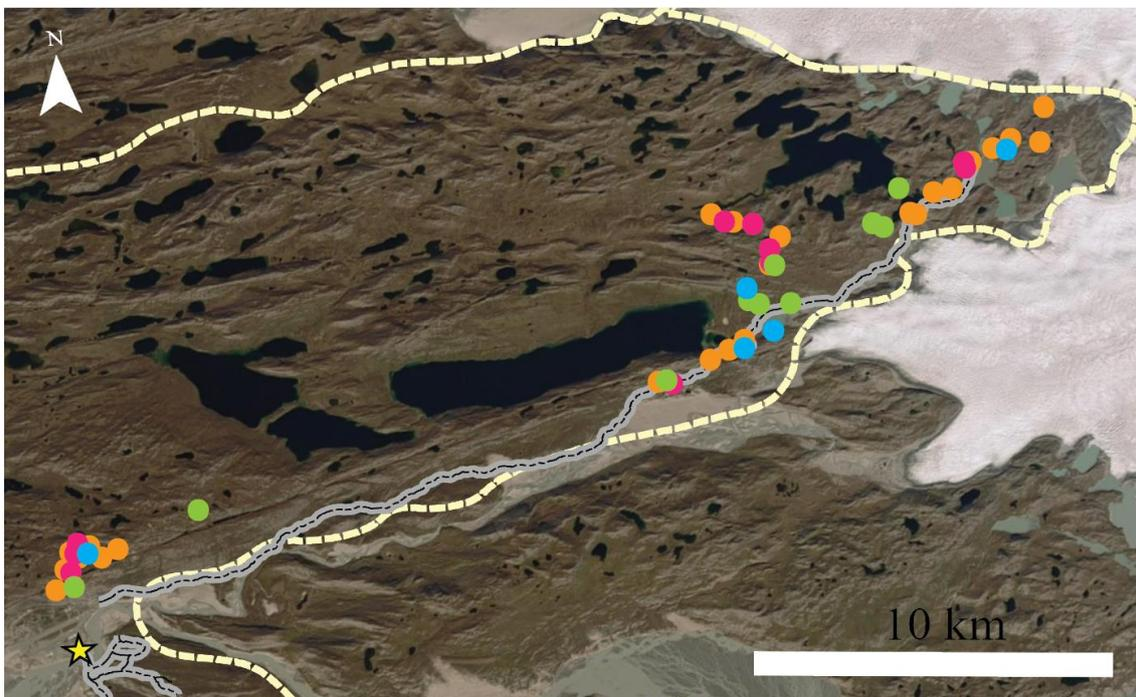
Figure 1. Satellite image overview of the sites visited in the field. Orange dots mark locations for glacial striation measurements, pink dots mark the location where cross-divide channels were visited, blue locations show polygonal terrain where UAV data and/or depth to ice estimations were acquired, and green dots mark the location of possible drumlins. Background image data credit: Airbus/Maxar Technologies/ CNES/ USGS – Google Earth.
