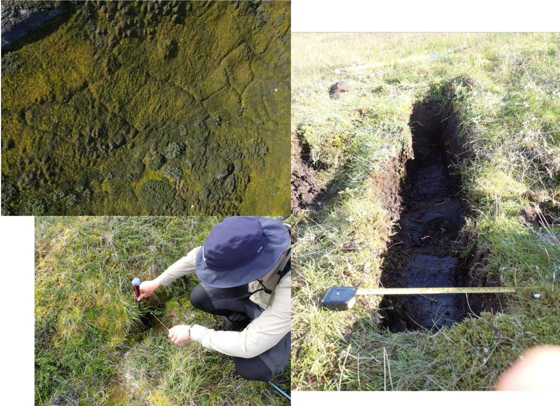
*Figure 3. Polygonal sites. Top left: UAV-borne image of polygonal sites (each polygon is ~ 4m across). Right panel: trench excavated to the ice layer on a polygon site, with the polygonal trough on the middle. Bottom left: steel pole measurement of depth-to-ice on a polygonal trough.*
